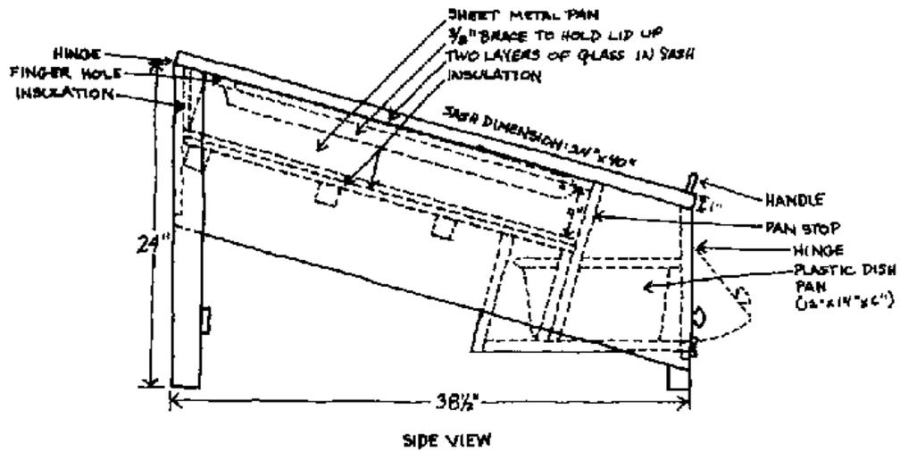
The wax melter has a double layer of 1/2" Celltex, except for the top rear, which has a single layer, and the front, which has no insulation.
